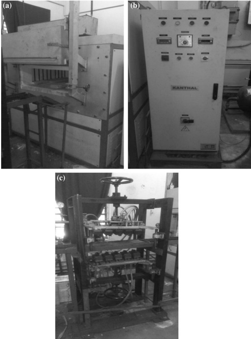
Fig. 30.1 a Closed chamber type furnace, b furnace control panel, c the nozzle bank setup, d the air compressor, e the compressed air flow circuit with digital flowmeter, f the test MS plate with eight thermocouples
